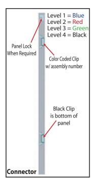
Each component has 2 clips, the lower clip is ALWAYS black. The top clip is color coded to distinguish which level. The color coded clip also contains the numbered
