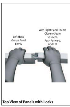
The first level of components contain pane locks that are located at the top of the panel for extra stability and seamless connection. When disassembling panels twist top connection slightly and lift right panel upward.
