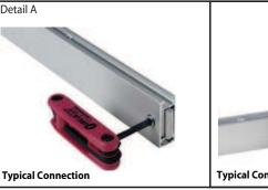
Most horizontal extrusion connections have a patented expandable lock. This lock inserts into the groove of an opposing extrusion. Tightening the lock with the Hex Key Tool expands the lock and creates a strong positive connection.
